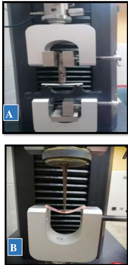
Figure (1) A- Transverse Gester machine, B- Transverse Testing Specimen on GESTER Machine
