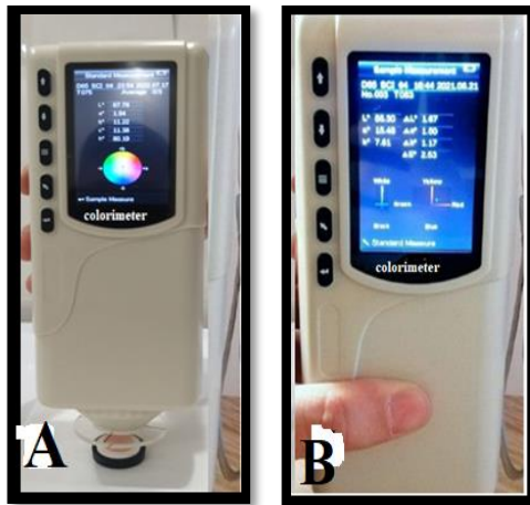
Figure (1): A. colorimeter device during initial reading; B. colorimeter devices automatically presented the transluency value ( \Delta E ).
