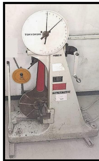
Figure (4): Charpy impact tester for impact strength measurement.
