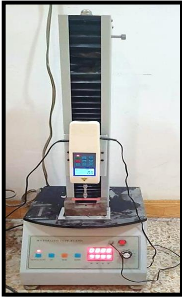
Figure (2): Universal testing machine for flexural strength measurement.
