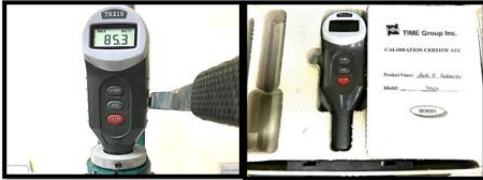
Figure (2): Shore D durometer hardness tester.
