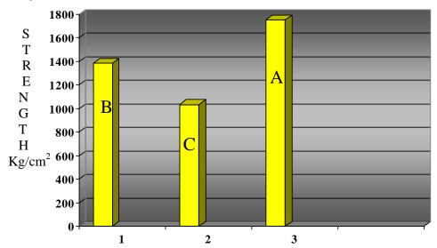
Figure (1): Duncan multiple range test for Rematitan Plus Investment. 1 : Mixed with tap water; 2: Mixed with distilled water; 3: Mixed with special liquid.
