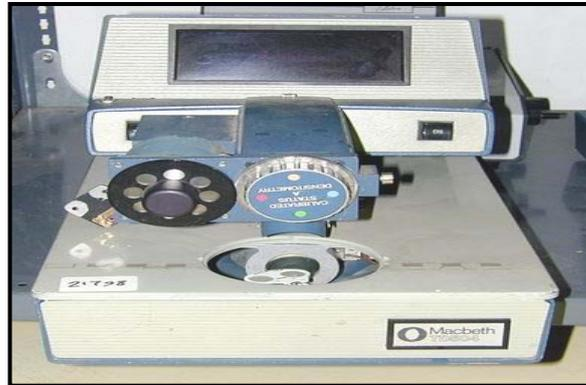
Figure(2): Densitometer Instrument
