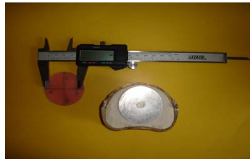
Figure (1): Aluminum disk flaking and acrylic resin specimen measurement with digital caliper
