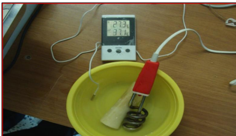
Figure(1): Thermostat-controlled bath containing physiologic saline.
