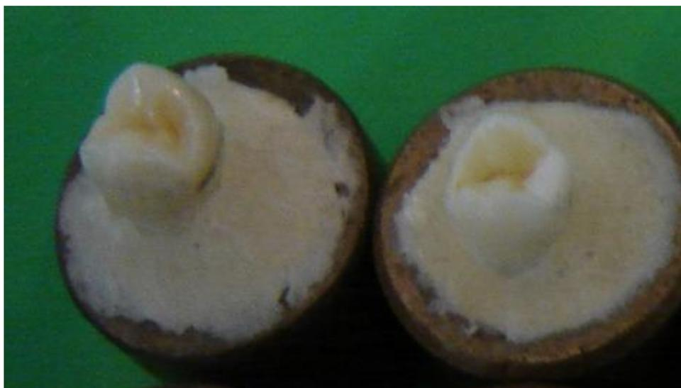
Figure (1): Test sample teeth fitted vertically into a metal cylinder filled by acrylic resin.
