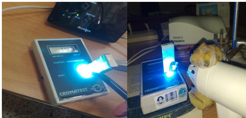
Figure (1): Light cure [BlueLuxcer™ (M–855) and Astralis 5–VIVADENT ] testing by a curing radiometer CROMATEST (7041).
