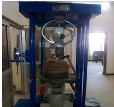
**Figure (3):** Universal testing machine(Instron)
