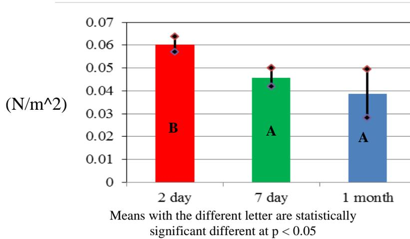
**Figure (4):** Mean  $\pm$  SD and Duncan's multiple rang test of tensile strength for EDTA
