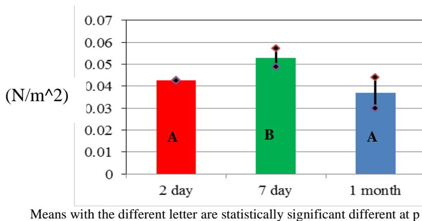
**Figure (6):** Mean  $\pm$  SD and Duncan's multiple rang test of tensile strength for (Corega)
