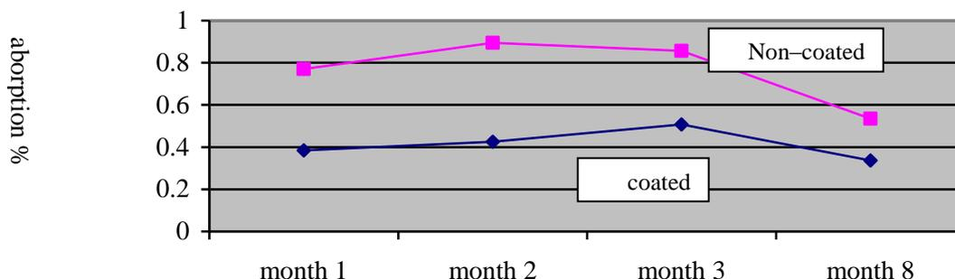
Figure (1): Percentage absorption of coated and non-coated soft liner
