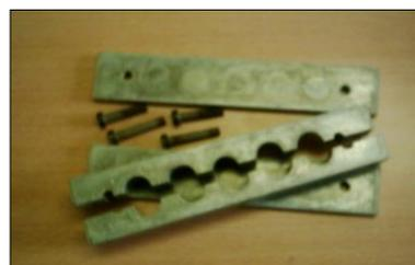
Figure (2): Split Metal Mould for preparing acrylic cylinder.
