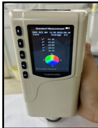
Figure (2): Colorimeter portable device for color change measurement
