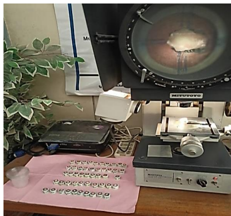
Figure (4): Surface roughness measuring of the teeth samples by profilometer
