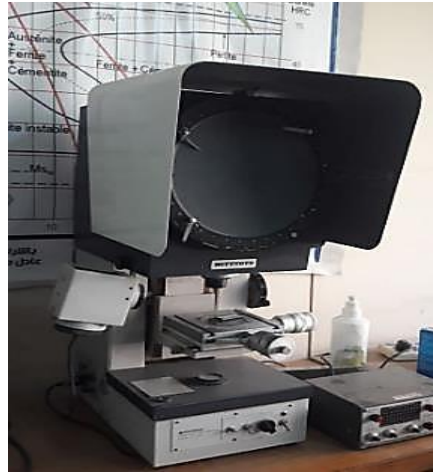
Figure (3): Profilometer (profile projector).
