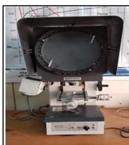
Figure (4): Enamel Surface Sample Measured by Using a Profile Projector.
