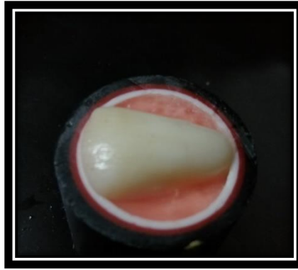
Figure (1): Bovine tooth specimen embedded in acrylic mold
