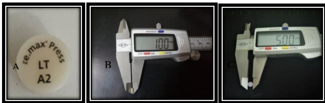
Figure (2): A: Ingot of E-max press ® ; B: Measuring the thickness of ceramic discs using digital caliper, C: Measuring the diameter of ceramic disc.
