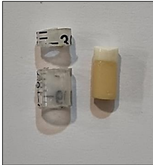
Figure (1). Glass ionomer with flowable composite as one sample and the adjacent rings that are used for preparing samples.
