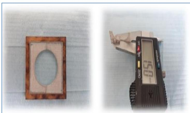
**Figure (3):** Gauging the thinness of the ring mold used for sample planning.
