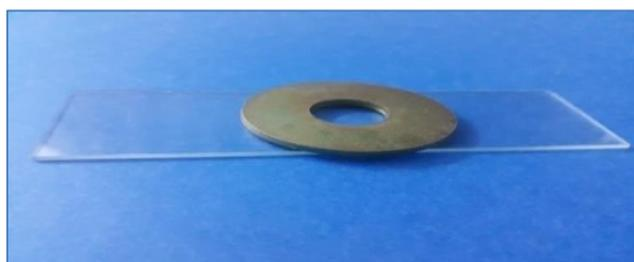
**Figure (1):** Ring of stainless steel mold located on a slide of microscope.
