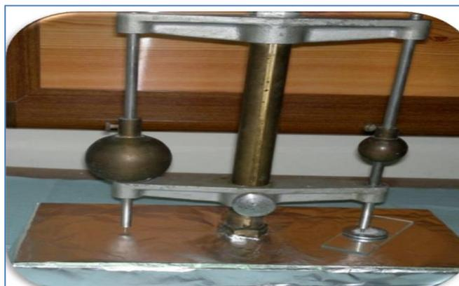
**Figure (2):** Gilmore needle device with the sample.
