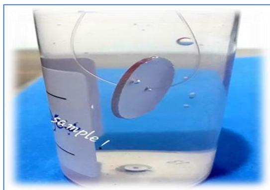
**Figure (4):** The model was suspended and fixed by nylon fiber.
