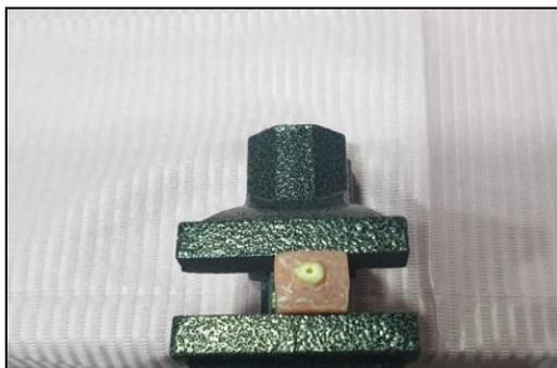
**Figure (1):** Fixation of acrylic block by bench vice.
