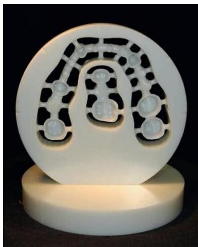
**Figure 5.** CAD/CAM interim fixed restorations milled from a resin disc. <sup>(6)</sup>
