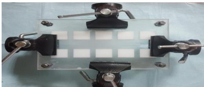
Figure (2): Parts of mold squeezed by screw, nuts, and G-clamps
