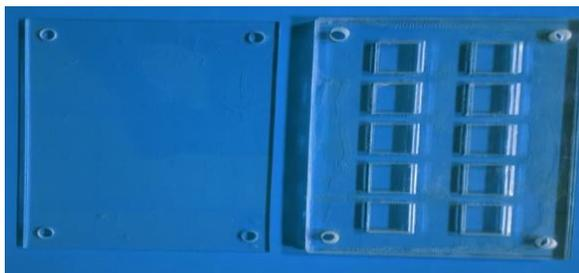
Figure (1): Acrylic plastic mold for the surface roughness test.
