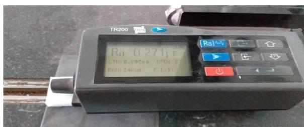
Figure (3): A portable surface roughness profilometer.
