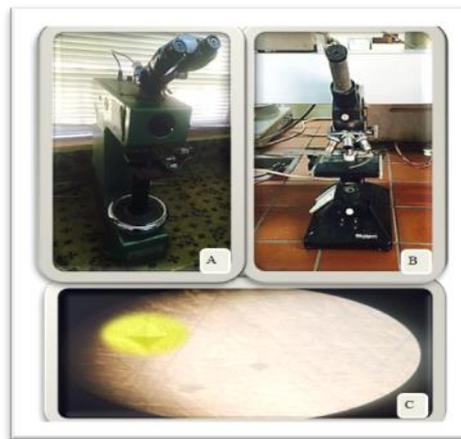
**Figure (3):** Surface Microhardness Measurement, (A) Vickers Microhardness Testing Machine, (B) Optic Microscope, (C) An Image of a Tetra Pyramidal Indentation Under Microscope.
