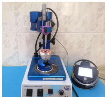
Figure (2): Diode laser hand piece stabilized by milling machine.
