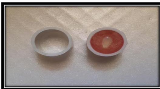
**Figure (1):** Teeth in a cold cure acrylic mold
